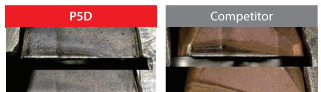
Wear comparison after 9m of drilling
