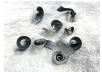
Cutting Chips of P3D
